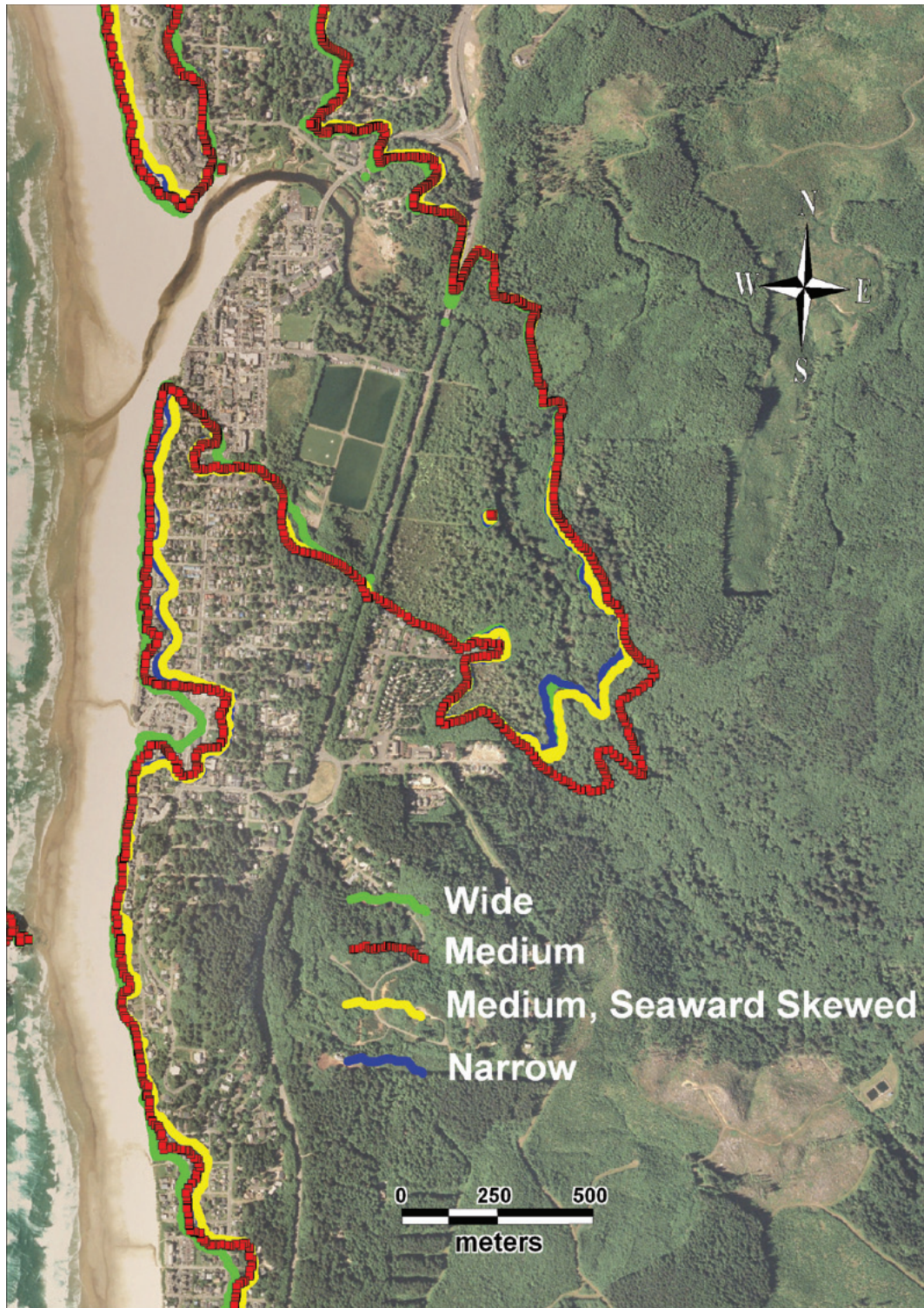
Figure 23. Difference at Cannon Beach, Oregon, between inundation for regional splay fault slip patch scenarios with differing rupture width and skew. All simulations use sources with "Average" fault slip of ~15 m. Simulations use an early numerical grid and early version of the SELFE hydrodynamic model, so inundations are significantly different from those used for the final inundation map but still useful for comparison. Medium = best-fit rupture width to geological data with symmetrical skew of slip ( q = 0.5 ); wide = medium rupture width plus 20 km; narrow = medium rupture width minus 20 km; medium seaward skewed = medium rupture width with q = 0.3 .
