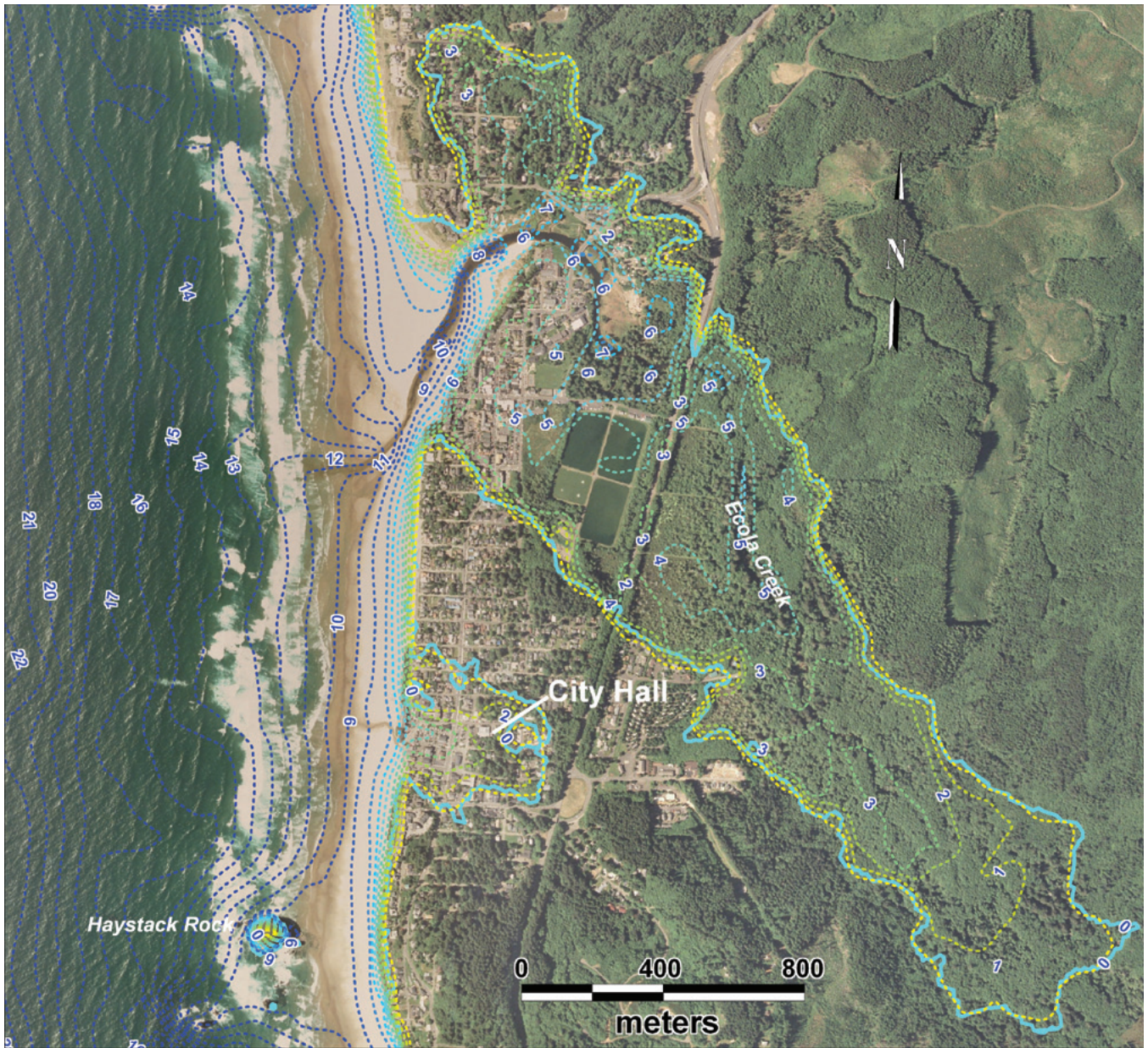
Figure 52. Maximum depth map for Average 14 scenario (preferred), approximating the ~70 percent confidence level for all variability in flow depth for Cascadia tsunami; contour interval (dashed lines) is 1 m; thick turquoise blue line is the maximum inundation for the Average 14 scenario.
